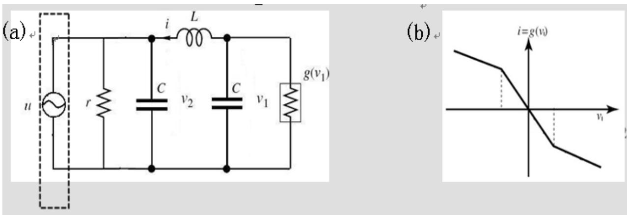
Figure 1: (a) The circuit diagram of the non-smooth BVP oscillator; (b) The  $v - i$  characteristics of the nonlinear resistor
