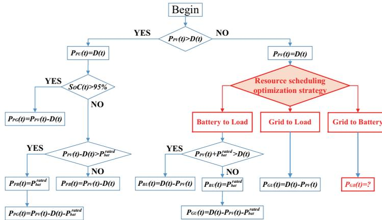
Figure 4: Framework of optimization of photovoltaic energy storage system
