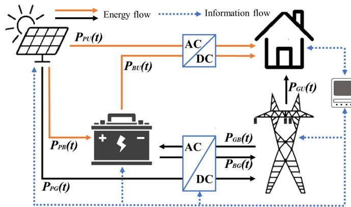
Figure 1: Grid-connected photovoltaic-battery system framework
