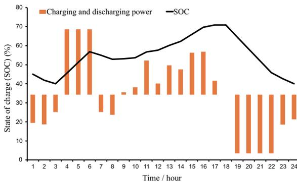
Figure 6: Charging and discharging power and SoC curve of energy storage system
