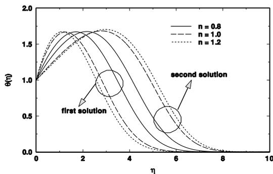
Figure 7: Variation of  $\theta(\eta)$  with  $\eta$  for several values of  $n$  with  $\alpha = -1.2$ ,  $Pr = 0.7$  and  $E_c = 1.5$ .
