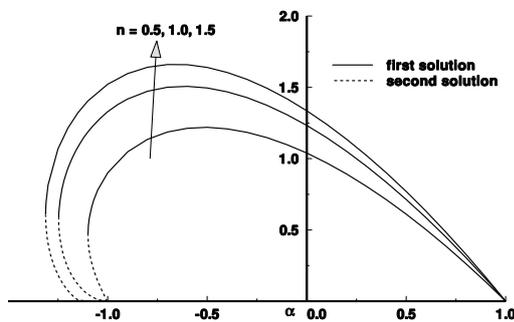
Figure 1: Wall shear stress  $F''(0)$  versus  $\alpha$  for different  $n$ .
