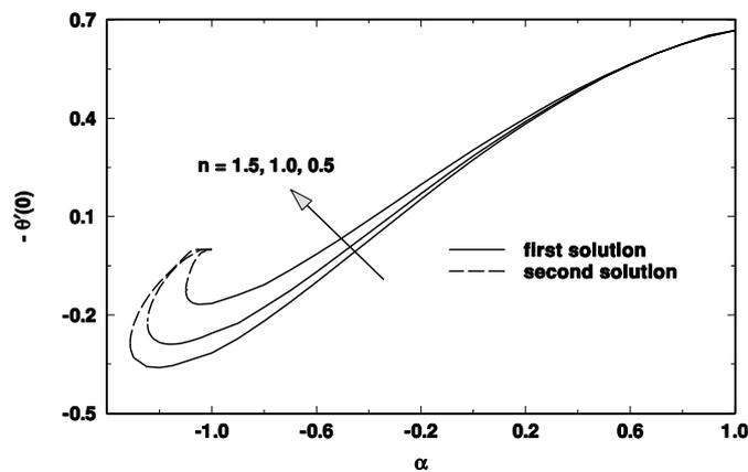
Figure 11: Variation of  $-\theta'(0)$  with  $\alpha$  for several values of  $n$  with  $Pr = 0.7$  and  $E_c = 0.5$ .
