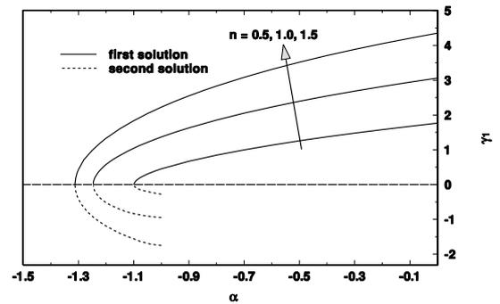
Figure 6: Plot of lowest eigenvalues  $\gamma_1$  as a function of  $\alpha$  for different values of  $n$ .
