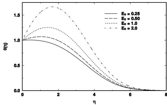
Figure 9: Variation of  $\theta(\eta)$  with  $\eta$  for several values of Eckert number  $E_c$  with  $n = 0.8$ ,  $Pr = 0.5$  and  $\alpha = -1.2$ .
