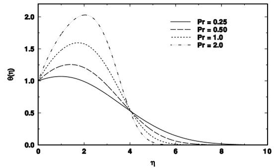
Figure 10: Variation of  $\theta(\eta)$  with  $\eta$  for several values of Prandtl number  $Pr$  with  $n = 0.8$ ,  $E_c = 1.0$  and  $\alpha = -1.2$ .
