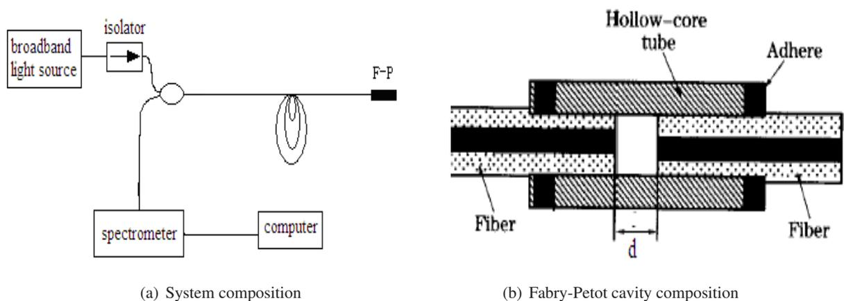
Figure 2: Demodulation system
