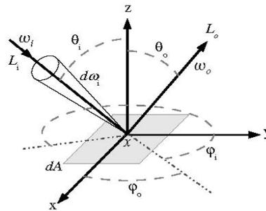
Figure 1: The bidirectional reflectance distribution function (BRDF) describes the ratio of outgoing radiance to incident radiance (irradiance).
