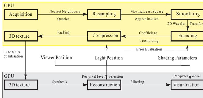
Figure 4: The GPU enhanced rendering pipeline.
