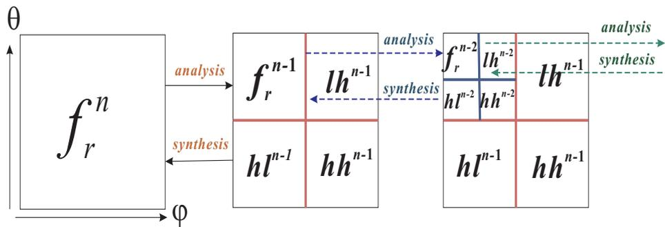
Figure 3: 2D Wavelet transform applied on each hemisphere of the original BRDF data.
